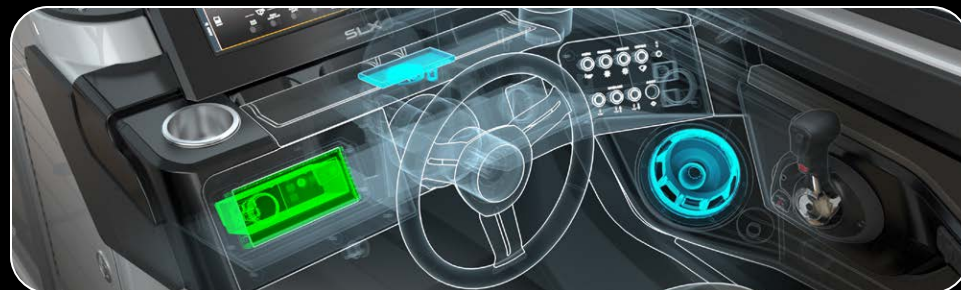
Fusion® Premier Audio system with Apollo™ RA770 stereo and inductive charging station
